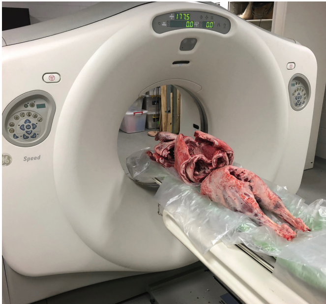
Image 2: Lamb cuts being CT scanned to measure LMY%
